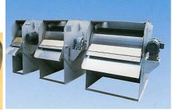
**Operation** Influent enters through a U-style head box where high flow velocities are minimized. The water with suspended solids flows under a baffle and then upward and is evenly distributed across the length of the screen cylinder. The screen is constructed of stainless steel wedge wire which can effectively handle grease, discrete solids without blinding.
